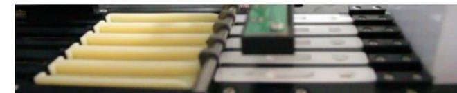
5. Patented cassette design protects test cards against humidity and makes reloading easier.
